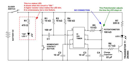
This schematic adds an optional LED that shows when the circuit is on. It is shown within the red square. It's completely optional.
