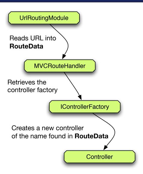
Figure 5.1: Controllers are created by the IControllerFactory based on a name inside the URL.
