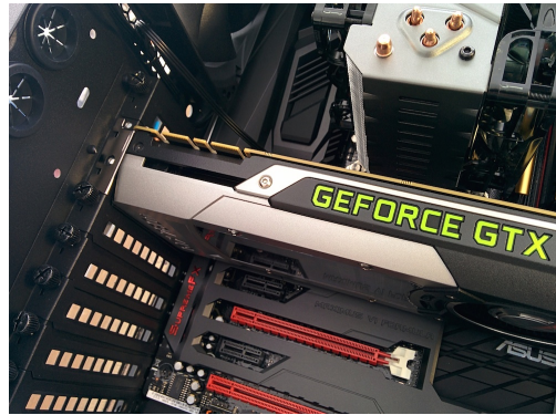
Figure 63—The GTX 780 Ti card mounted in the PCIe expansion slot on the motherboard
