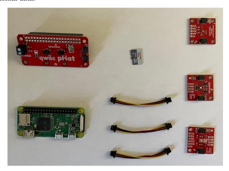
Putting together the sensor hub should feel like putting together a collection of Lego pieces. The Qwiic Connect HAT should slide nicely on top of the Raspberry Pi header pins, and from there you can daisy chain all the breakout boards together (in no particular order, as I2C doesn't dictate any particular orientation), as shown in the following picture.
