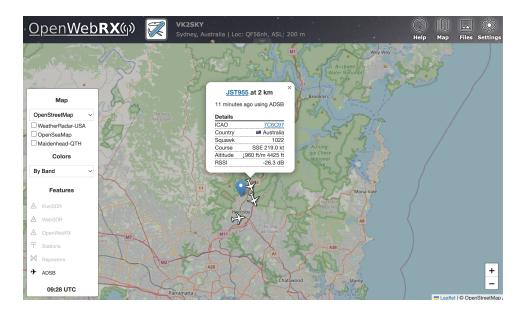
The Map display opens in a new browser tab, so we can see the movements of all detected aircraft on a display similar to commercial tracking web sites.
